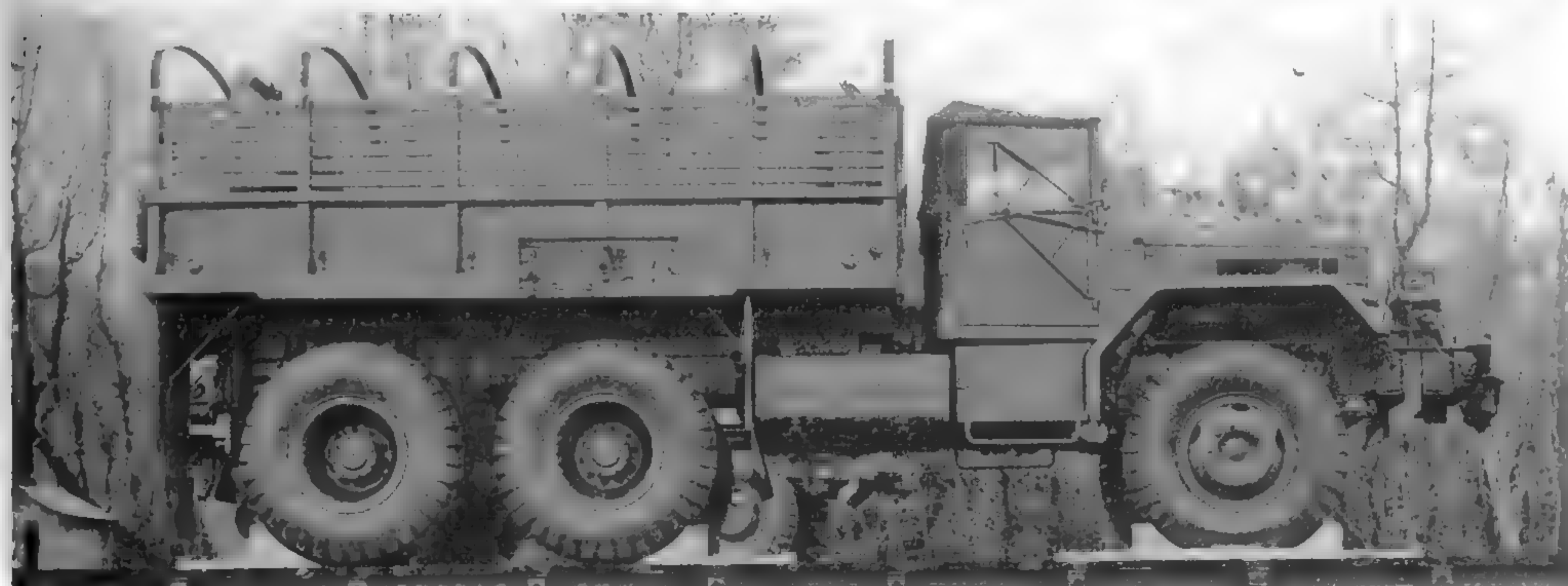
This huge M125 was photographed leaving Mack's Allentown factory via rail. The pioneer rack was mounted on the side of the cargo bed, and the powerful winch is visible behind the front bumper. (Photo courtesy of the Mack Trucks Historical Museum)
